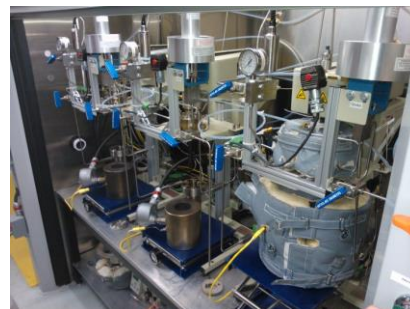
Three of our Autoclave Engineers Pressure Reactors with our H 2 (g) uptake measurement and data acquisition system.
